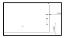
Step 2: Replace the magnet strip The magnet strips (+ screws) from the existing benches will be reused on the new benches. Make sure they are placed on the correct side of the bench, see the illustration above.
